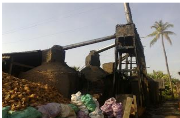
FIGURE 11: CHARCOAL MAKING KILN FROM COCONUT SHELL
