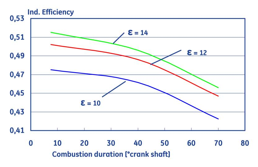
Higher compression-ratio helps the efficiency
