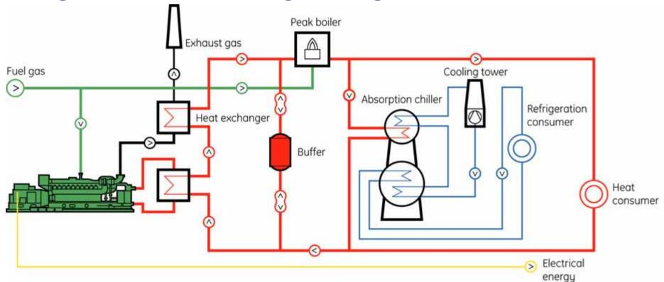
Electr. Output: 526 kW Recoverable Heat: 550 kW
