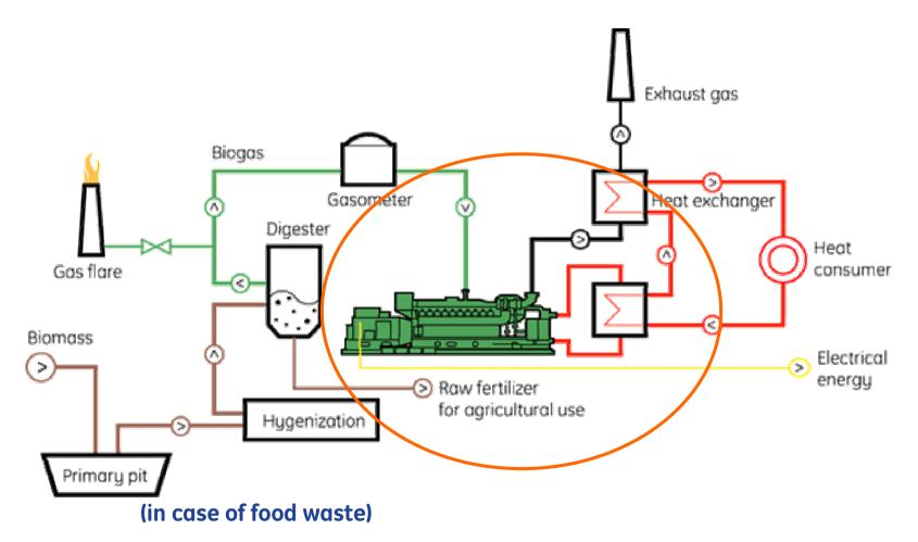
biogas-cogeneration units are core part of biogas plant, in combination with enhanced digester-technology
