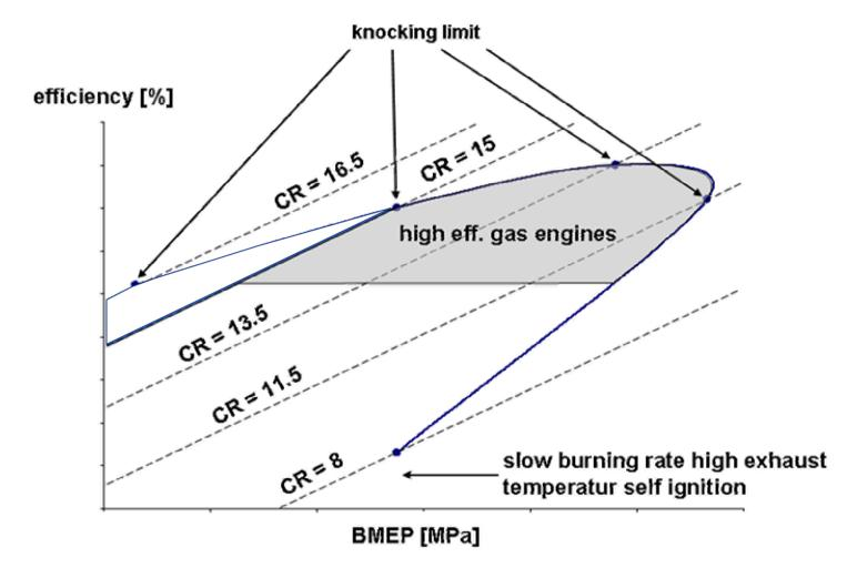
The optimum of compression ratio and BMEP must be found
