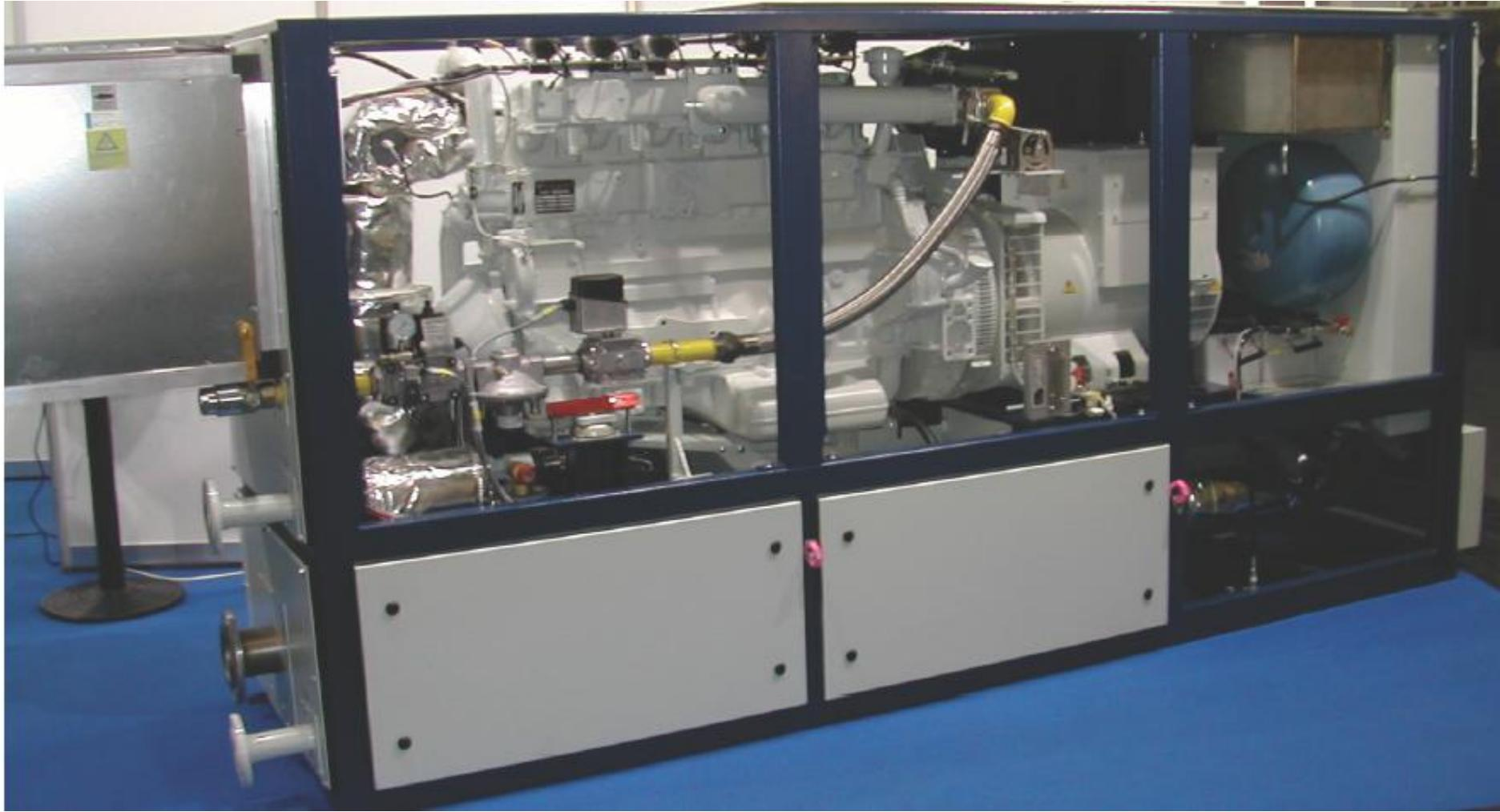
Co-gen package ca. 200 kW Co-gen 集装在大概200kW
