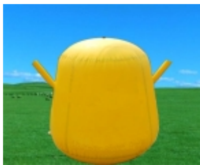
Figure 12: Partially Submerged Plastic Digester (basic form)
