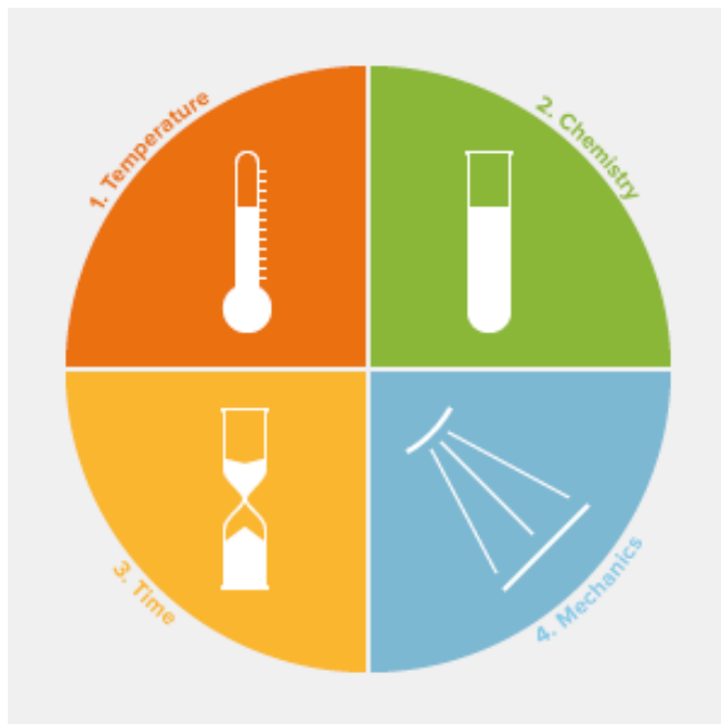
Figure 1: Sinner Circle, parameters of cleaning performance (In washing machines the mechanical action is provided by the drum, agitator or impeller movement).
