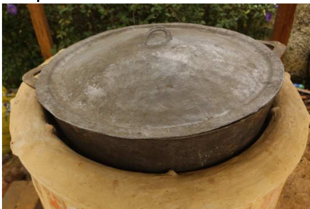
Pot sits “in chimney”, the 10 mm distance holders of the metal ring, define the space between stove and pot
