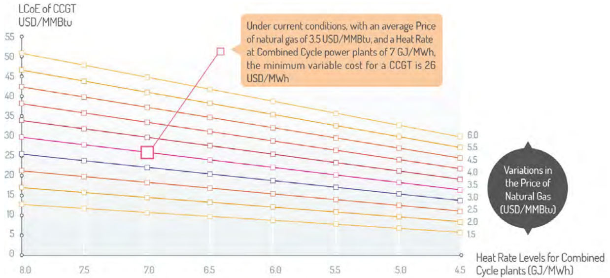
Figure 16. Analysis of sensitivity of the variable cost of a Combined Cycle plant (USD/MWh) due to changes in cost of gas (USD/MMBtu) and heat rate (GJ/MWh) - Source: CENACE, EIA.
