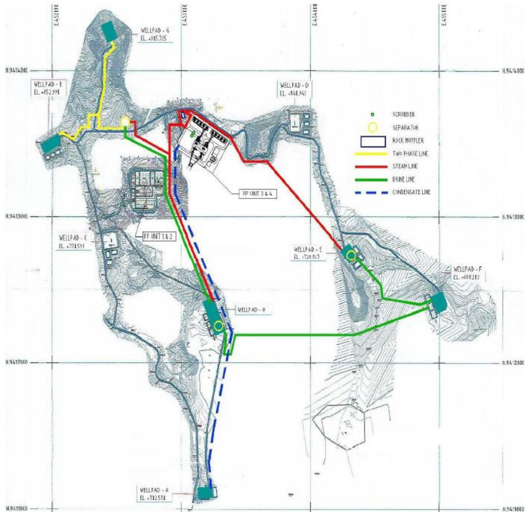
Figure A2.3 – General Layout for the Ulubelu 3&4 Development
