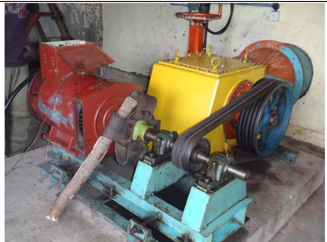
Photo 4: Turbine Wonorejo, wooden stick to keep system stopped, Oct 10
