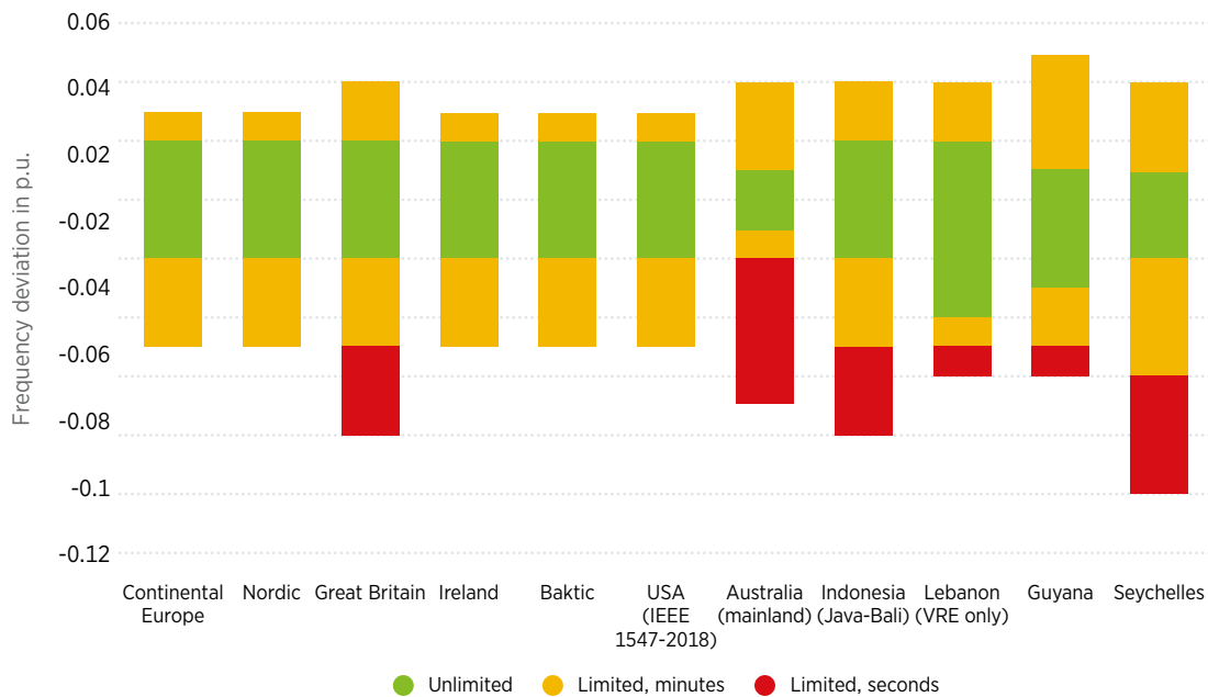
Figure 8 Frequency ranges required in grid codes in different synchronous areas of different sizes
