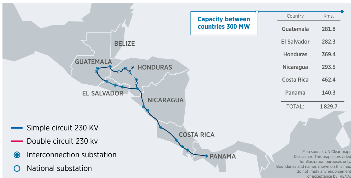
Figure 24 The Regional Electric System interconnecting Costa Rica, El Salvador, Guatemala, Honduras, Nicaragua and Panama
