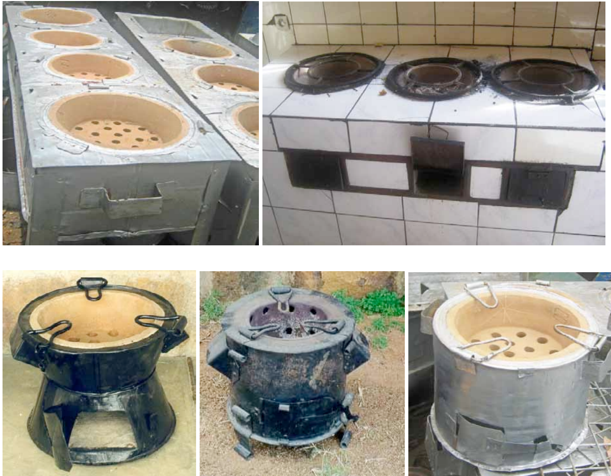
Fig 7: Different designs of improved institutional (top) and household (Below) charcoal stoves used in Kenya and Rwanda
