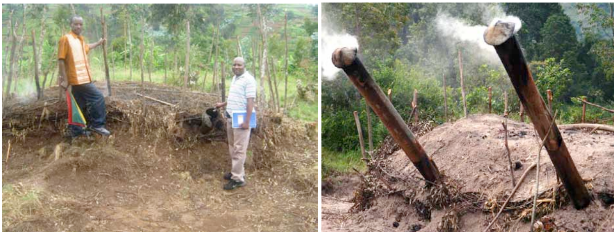
Fig 45: Earth mound kilns with chimneys to increase their efficiency in Nyamagambe, Rwanda. Source: Author
