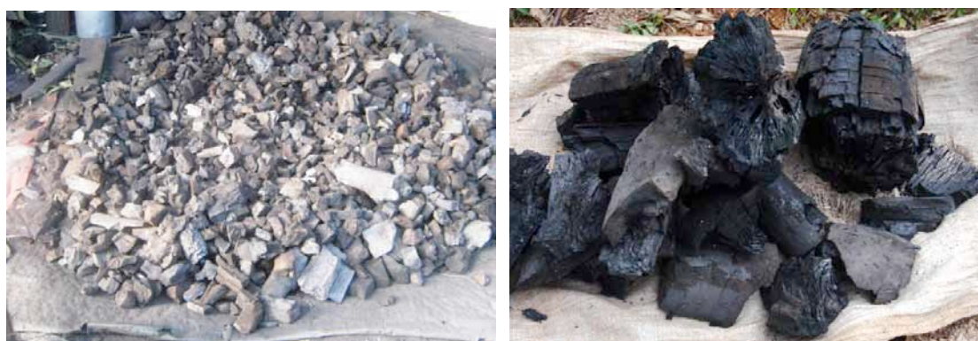
Fig 32: Poor quality charcoal from Pinus (Left) and good quality charcoal from Eucalyptus in Nyambugogo, Kigali.
