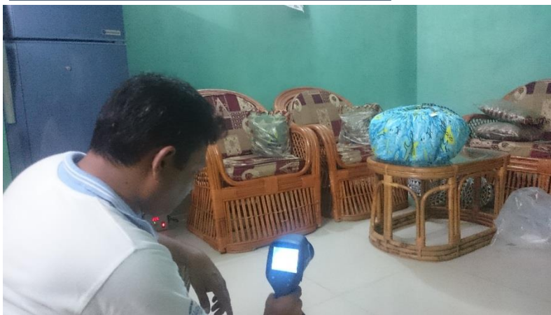
Figure 13: FLIR thermal camera used for heat loss measurement
