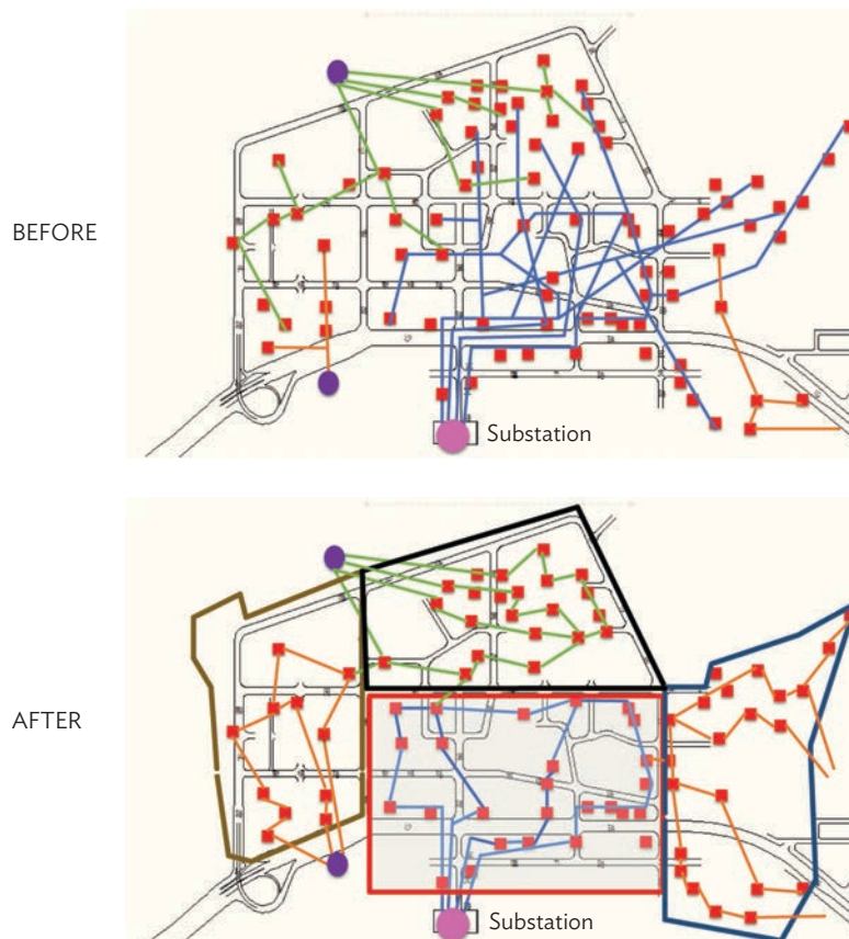
Figure 4: System Structural Enhancements Adopting Grid Partitioning Design
