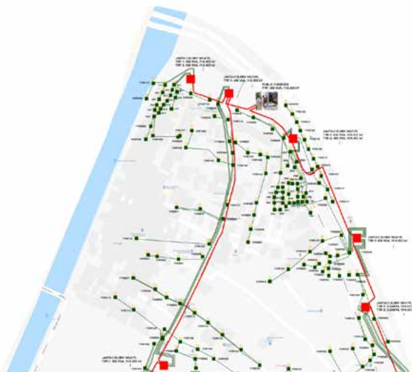
Figure 8.2.21: Janta colony distribution network with 1 public charger
