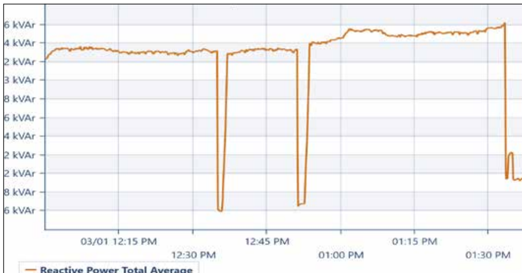
Figure 5.6.3: Three phase reactive power observed during EV charging period
