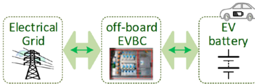
Figure 2.13: Off-board EVBC: G2V and V2G operation mode [53]
