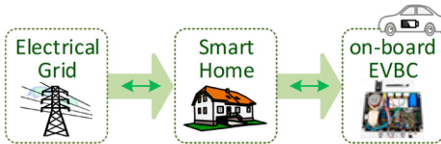
Figure 2.10: On-board EVBC: G2V and V2G operation mode [53]
