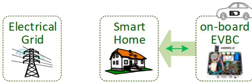
Figure 2.12: On-board EVBC: V2H operation mode [53]
