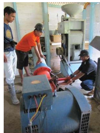
Photo 27: Direct-drive, productive end-use
