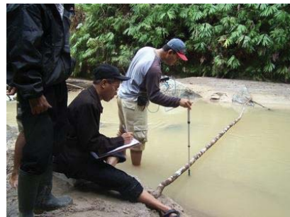
Photo 15: Flow measurement, Lembung, Sulawesi
