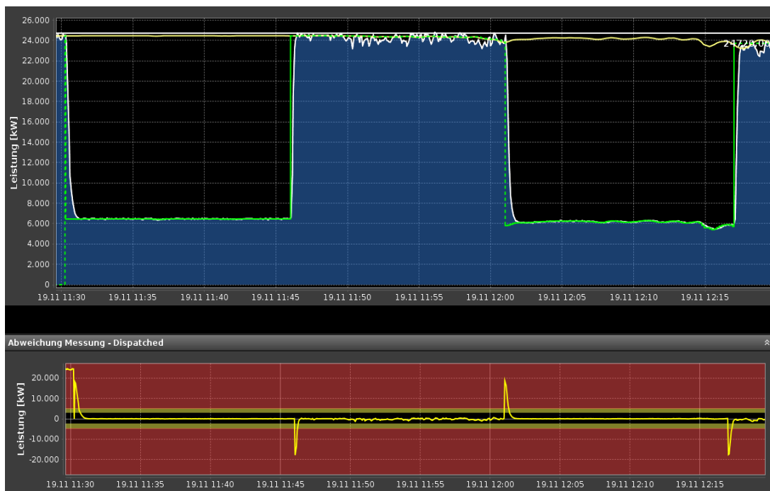
Figure 28: Virtual Power Plant curtailing wind park to provide ancillary services to the system operator.
