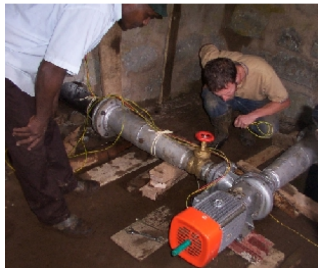
The induction motor as generator produces 2.2kW but a shaft extension provides a 3kW drive for mechanical loads.
