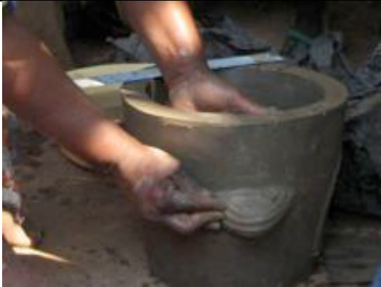
Half moon shaped handles are better than round knobs to prevent stove from tipping over
