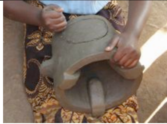
cut the door after one day and fit a knob
