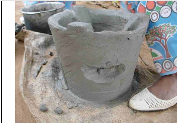
make holes in the wall to fit the handles right through the wall, so they don't break off
