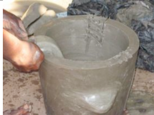
fix potrests properly and make sure that they go straight down inside
