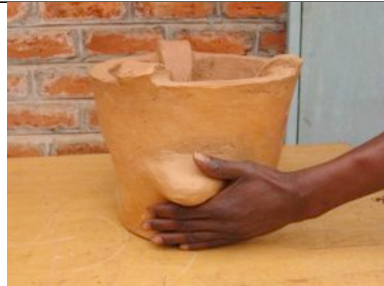
Handles must be opposite each other and not too low above floor (one palm width)
