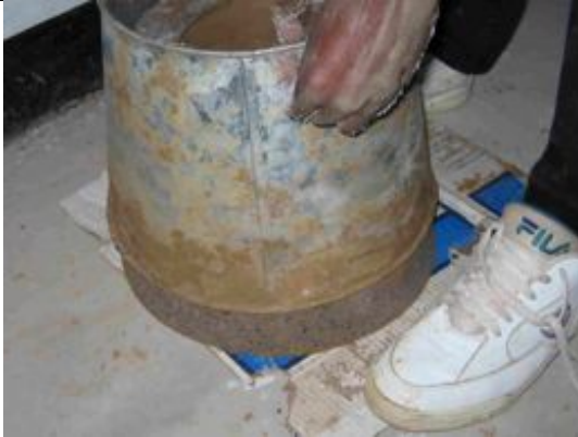
get the stove out of the mould
