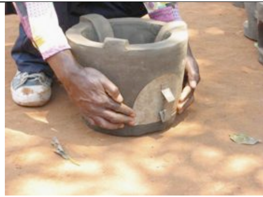
Take a ruler to find centre of stove. Then draw the door by using the door mould on one side.
