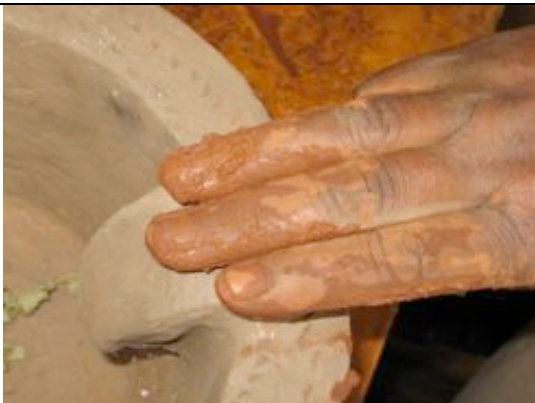
Potrest width should be 3 fingers
