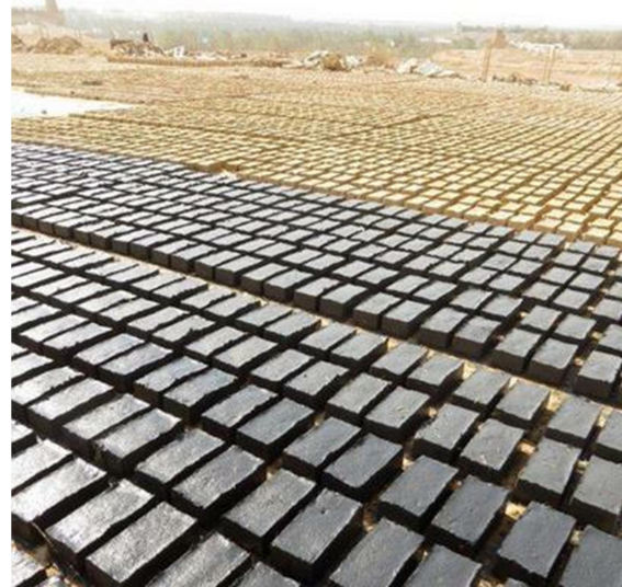
Figure 3.15: Standardized mud blocks production in Saudi Arabia – Source: www.theconstructionindex.co.uk/
