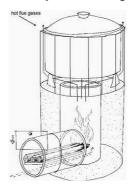
There is a 'skirt' around the pot. This skirt, and the pot hole, are customised to the outer pot diameter, which is controlled by cooking capacity of the pot.
