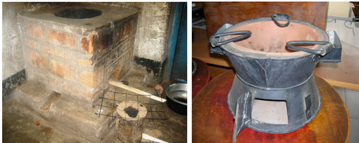
Fig 46: Efficient Rocket stove for firewood promoted by GTZ (Left) and Kenya Ceramic Jiko for charcoal which has had high adoption rate in Kenya. Source: Author
