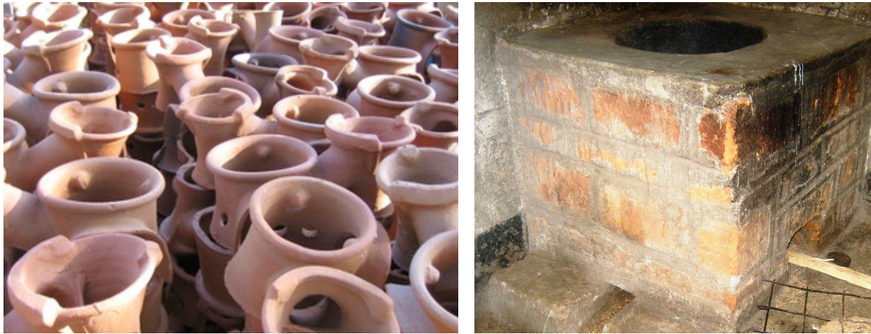
Fig 3: Anagi wood stove from Sri Lanka (left) and Rocket stove used in Kenya and Uganda Source: www.hedon.info/StoveImages and Author
