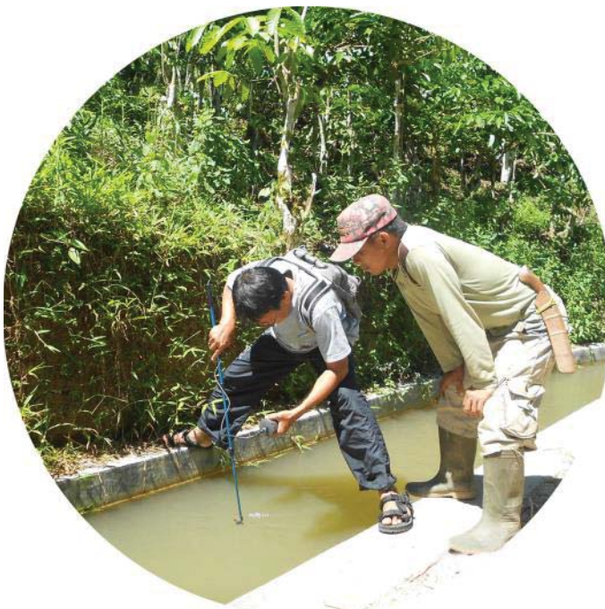
Measuring water flow in the channel using current-meter.
