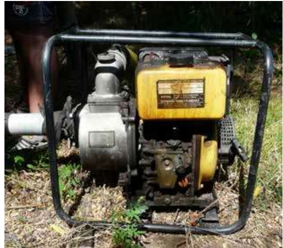
Old diesel pump
