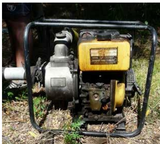
Old diesel pump
