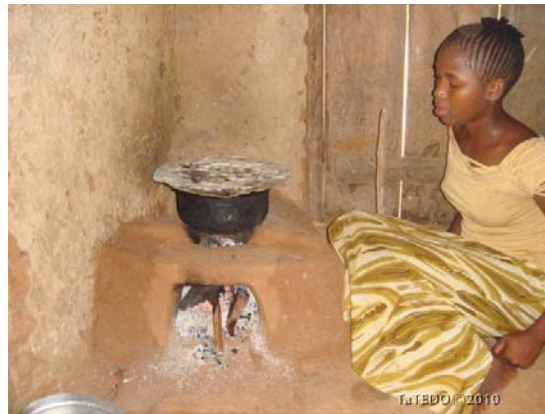
A woman in village cooking with Improved Firewood Saving Stove (Ukombozi Stove)
