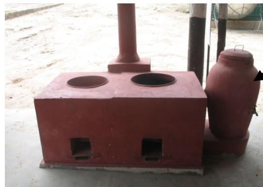
Multifunction, brick made okoa fuel wood stove with water heater.
