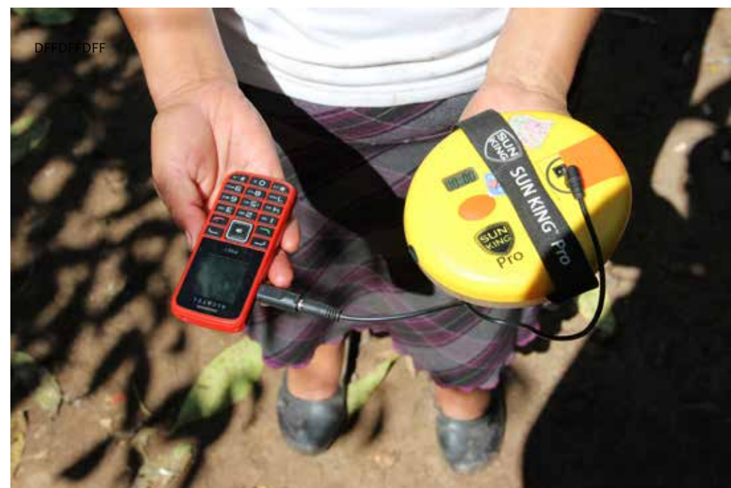
A pico photovoltaic system can be used to recharge cell phones.
