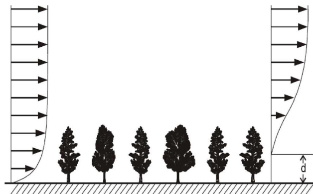
Figure 3.129: Wind shear due to roughness
