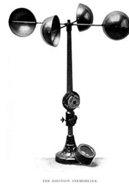
Figure 3.130: A hemispherical cup anemometer as invented in 1846
