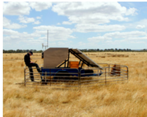
Figure 3.133: Wind monitoring using the Fulcrum3D SODAR
