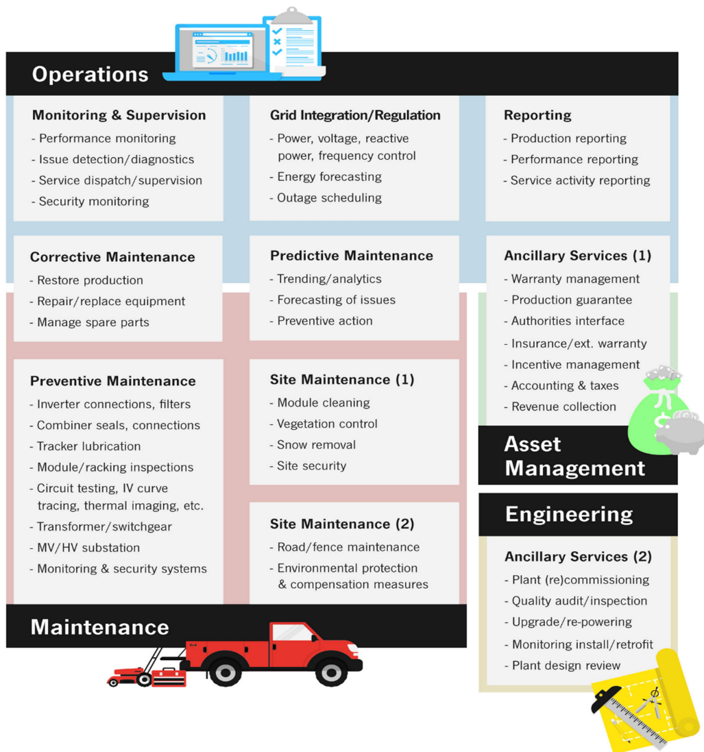
Figure 4.42: Example of O&M action point of a solar PV power plant
