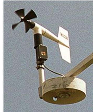
Figure 3.132: Helicoid propeller anemometer incorporating a wind vane for orientation
