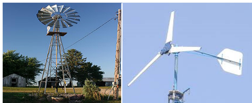
Figure 3.148: High-solidity turbine (left) and low-solidity turbine (right) – Courtesy: Wikipedia
