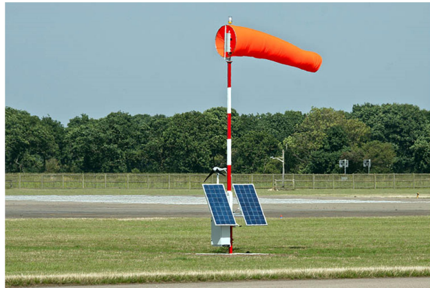
Figure 3.134: Windsock with solar-powered data capture device
