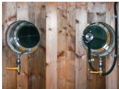
2 bull's eyes with wipers, wash nozzle and lamp built into the fermenter
