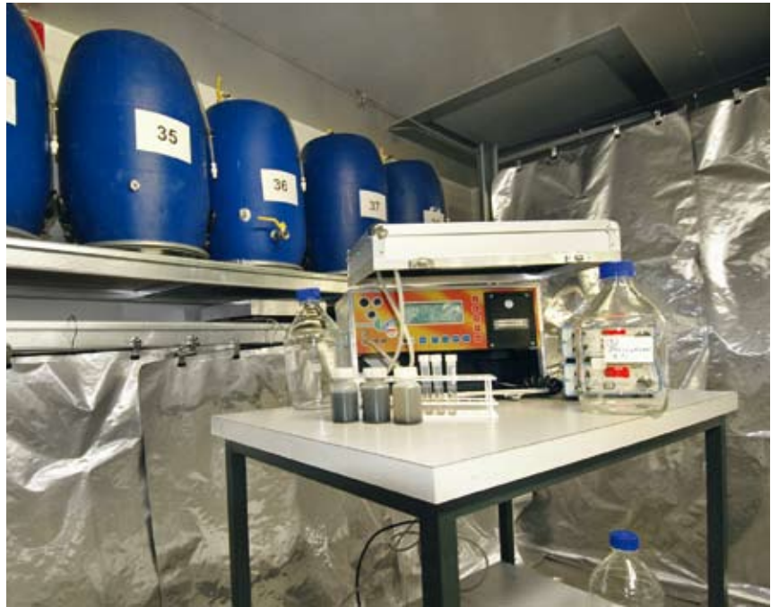
A system with 70 batch fermenters allows extensive research in the field of biogas production.
