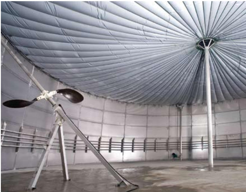
Internal view of a stainless long arm agitator, submersible agitator and double-membrane roof
