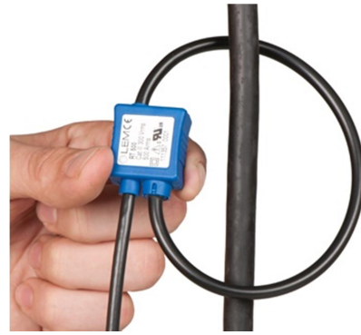
Figure 6.40: Flexible Rogowski coil for electrical current measurements
