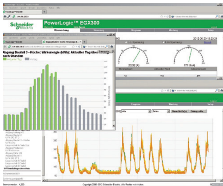
Figure 6.71: Screenshot of a typical EnMCT software showing basic dashboard functions with actual consumption profiles in different time scales
