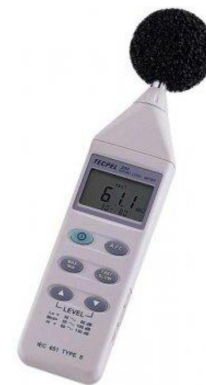
Figure 6.54: Typical noise meter
