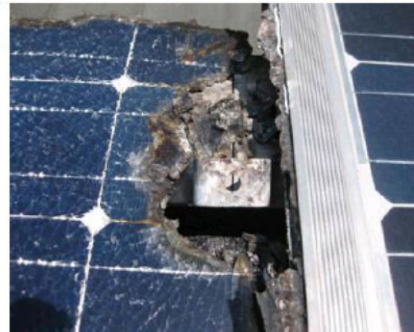
Broken cell, similar behavior as a shaded cell
