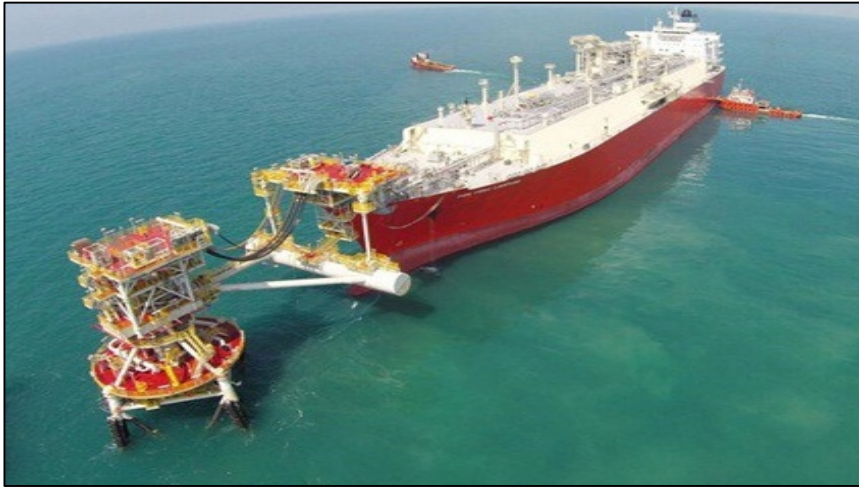
Figure 10 – Tower Yoke Mooring in Indonesia
