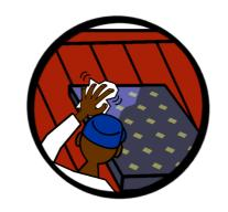
From time to time, check the condition of the modules. If they are dusty or dirty, carefully wash the modules' top glass surface using water and a soft cloth.
