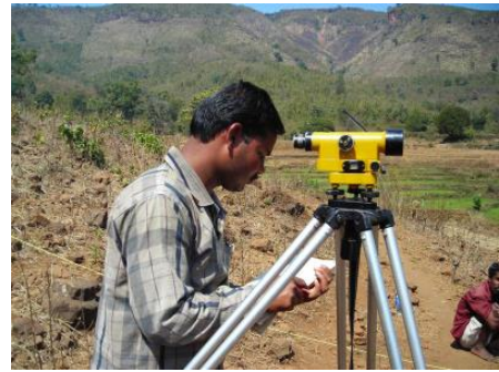
Figure 2.20: An engineer taking readings from a dumpy level
