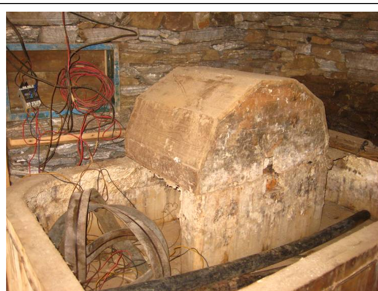
Mixing drum for the raw materials to produce paper.
