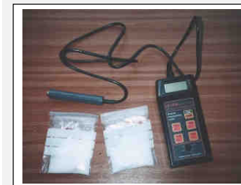
Figure 7-7 Portable conductivity meter and carefully weighed bags of salt
