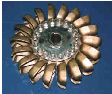
Figure 8-5 Locally Manufactured Pelton p.c.d.180 mm (Sri Lanka)
