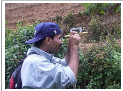
Figure 7-3 Head measurement using an Abney Level in Nepal
