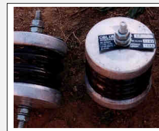
Figure 16-1 Spark gap lightning arrestors
