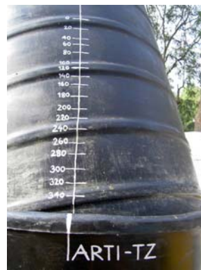
Figure 14: Scaling on gasholder
