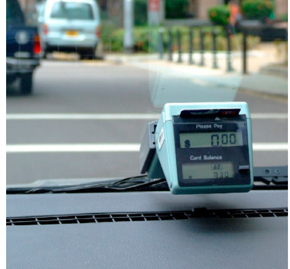
Figures 22a, b Electronic Road Pricing Gantry (left) and on-board system for fare collection (right) in Singapore.
