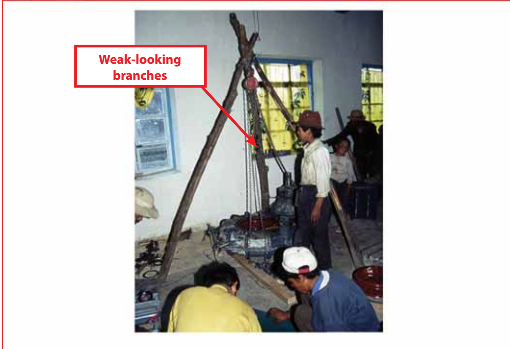
Three tree trunks – tied together as a tripod – look rather weak
