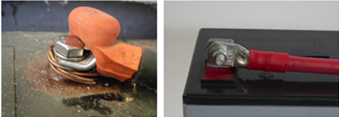
Figure 6.10: Poor connection (left) and good connection (right)
