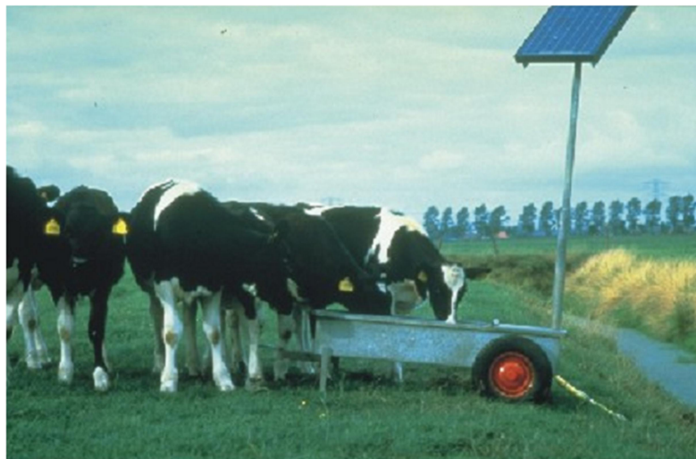
Figure 1.20: A DC solar pump powered by solar panels to bring water to grazing cattle in the field – Courtesy: Prof. Dr.-Ing. Habil Ingo Stadler
