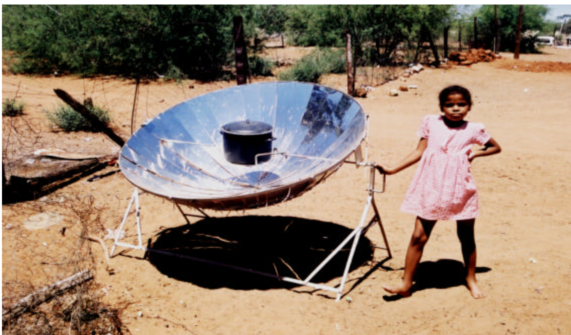
Figure 9 The SK12, the most efficient solar stove model during the social acceptance test
