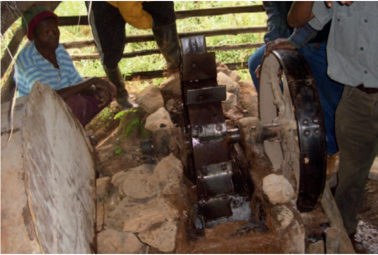
A maize mill before its refurbishment made of junk metal pieces.
