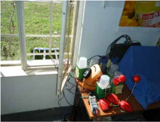
Figure 1: Various solar lamp models for test-charging in the GIZ office in Arua.
