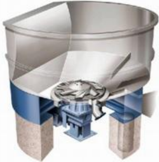
Pulper, swim-sink separation 浮渣破碎 沉积分离
