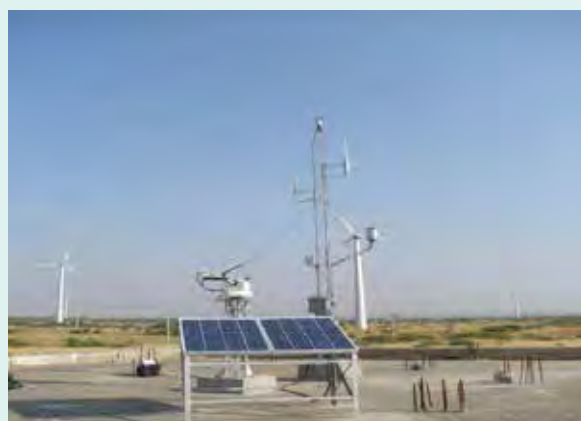
An illustrative SRRA station with solar radiation and ambient meteorological parameters sensors.
