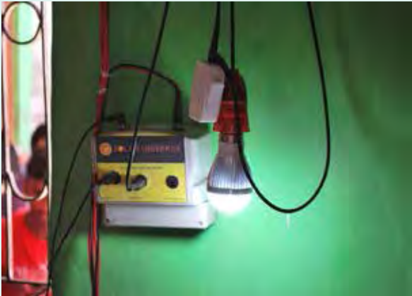
DC home system with LED bulbs, mobile charging kit and table fan in Khoiri Village, India.
