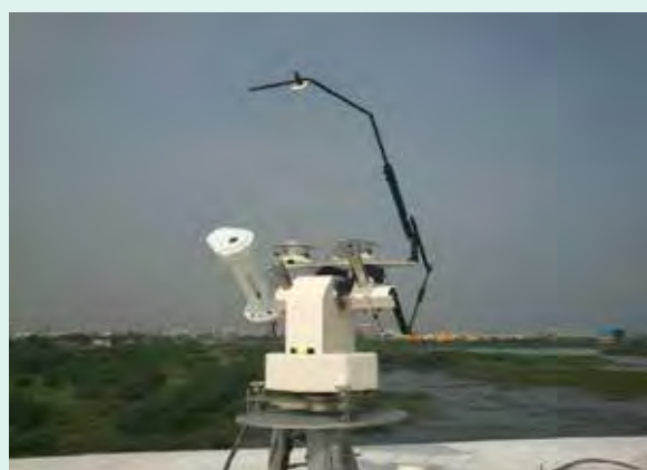
The 2-axis solar tracker with a pyrheliometer, an absolute cavity radiometer, a pyranometer and a shaded pyranometer
