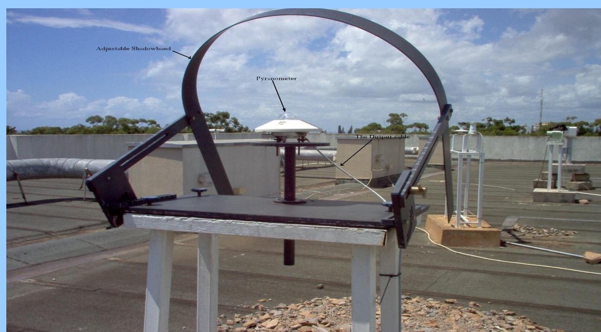
Figure 1 shows a photograph of a precision spectral pyranometer (PSP) fitted with a shadowband. It measures the diffuse component of solar radiation. It is on field operation at the Eduardo Mondlane University (UEM).
