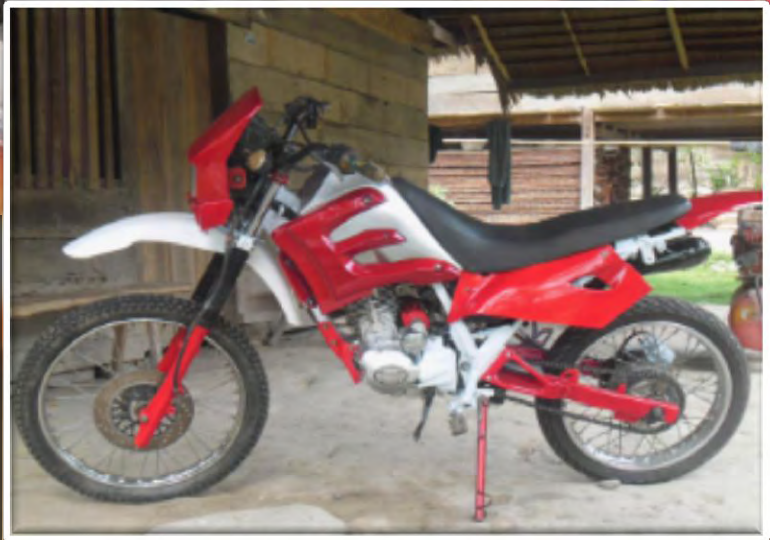
Motorbike modification in Tandung, West Sulawesi. Normal motorbike ride to Masamba takes up to 4 days. By improvising the motorbike suspension, the distance can be covered in 2 days. Such modification was usually done in Masamba, 30-40km from the village. The workshop also does spray painting work.
