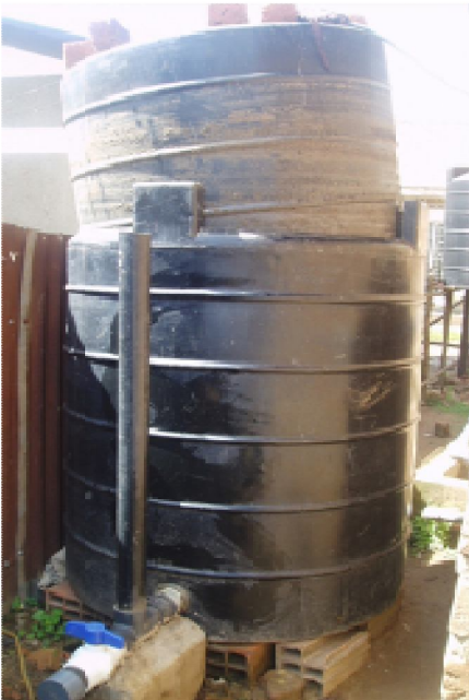
Picture 7 and 8: Examples of floating drum biogas digesters. On the left side, digester made out of poly-ethylene tanks and on the right side constructed with bricks and steel.
