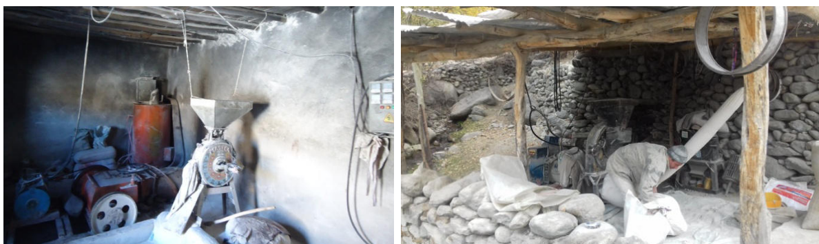
MHP 4114, productive end-use, possibility to connect a flour mill via a V-belt to the turbine
