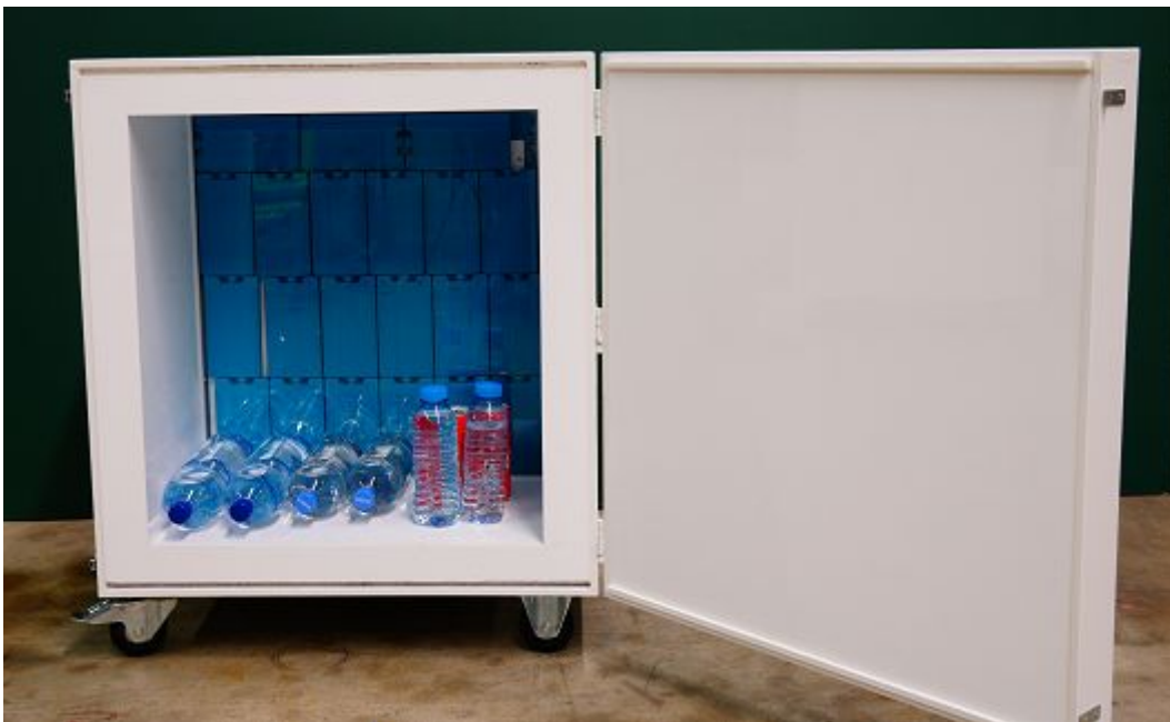
Figure 19: DDR with ice packs in the back wall around the evaporator
