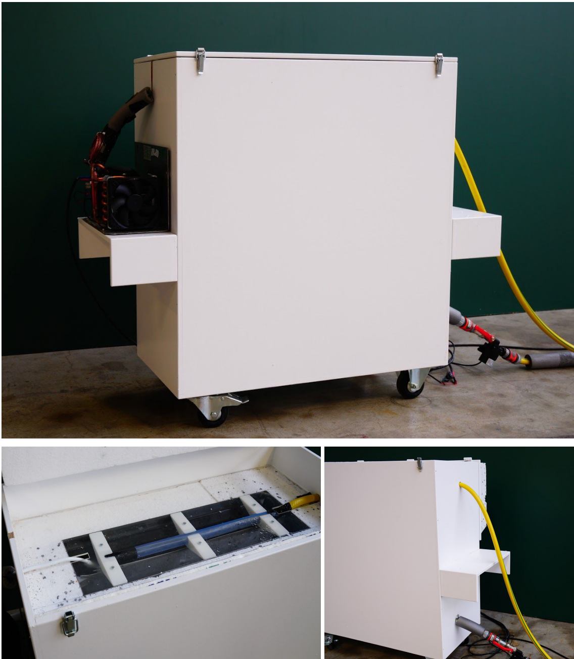
Figure 26: Water chiller based on ice storage with cooling unit (u), the water distribution tube above the ice block at the evaporator (d.l.) and tubes for the external water circle (d.r.)
