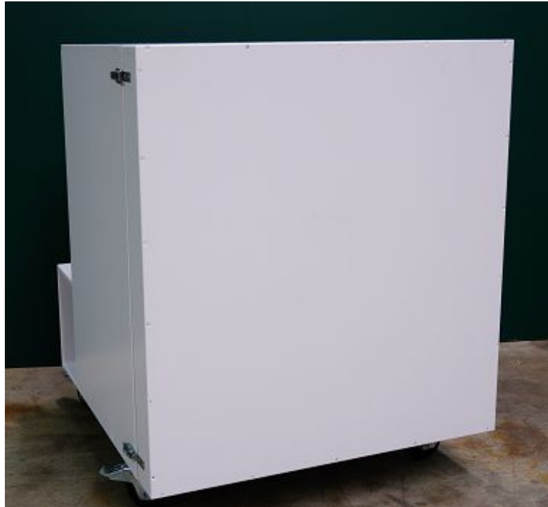
Figure 18: Painted wooden box of the direct drive refrigerator (DDR)
