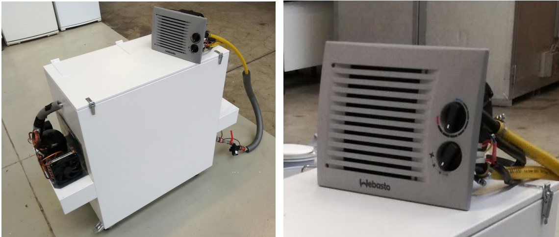
Figure 31: Cooling room application with an air heat exchanger
