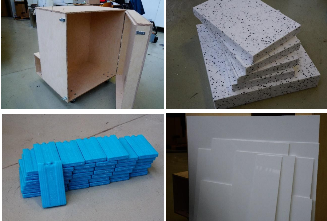
Figure 23: Wooden box (u.l.), polystyrene insulation material (u.r.), ice packs for ice storage around the evaporator (d.l.) and the acryl glass plates for the internal covering
