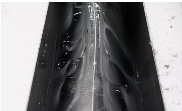
Figure 34: After 24 h ice formation process at the given experimental setups (see Table 3) an ice block of around 26 - 28 kg was formed
