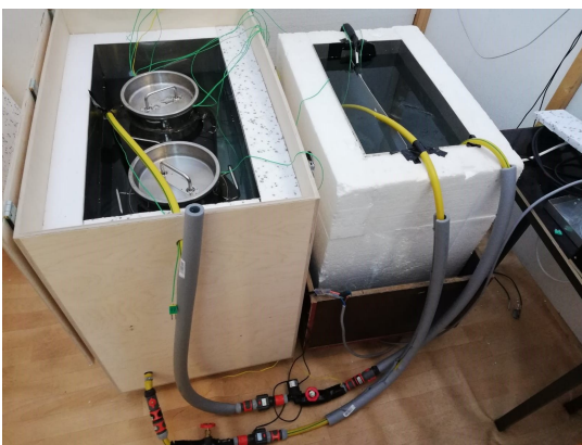
Figure 38: Experimental setup for testing the water bath application of the water chiller to cool down milk with the given settings (see. Table 5).
