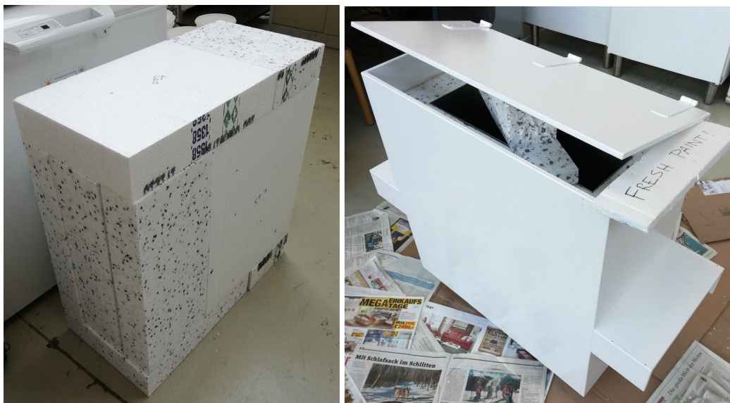
Figure 30: Cut insulation material for the ice storage (l.) and the painted wooden box with the integrated insulation material and metal box (r.)
