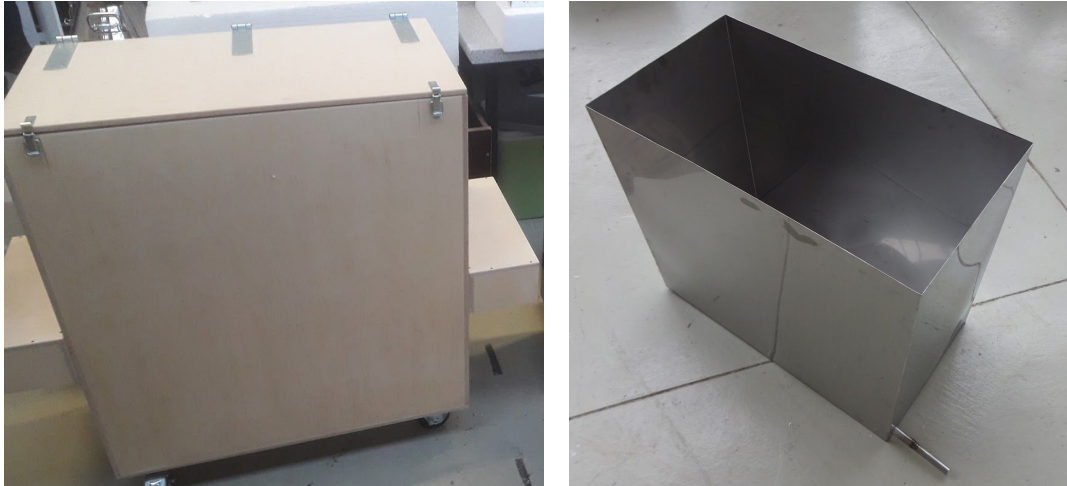
Figure 29: Wooden box (l.) and metal water container (r.) of the water chiller
