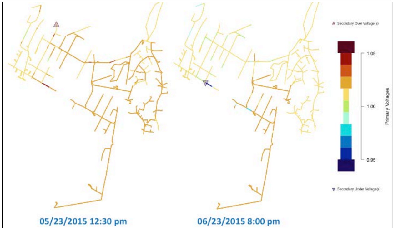
Figure 30. May 23, 2015, highest (left) and lowest (right) voltage heat map for feeder L
