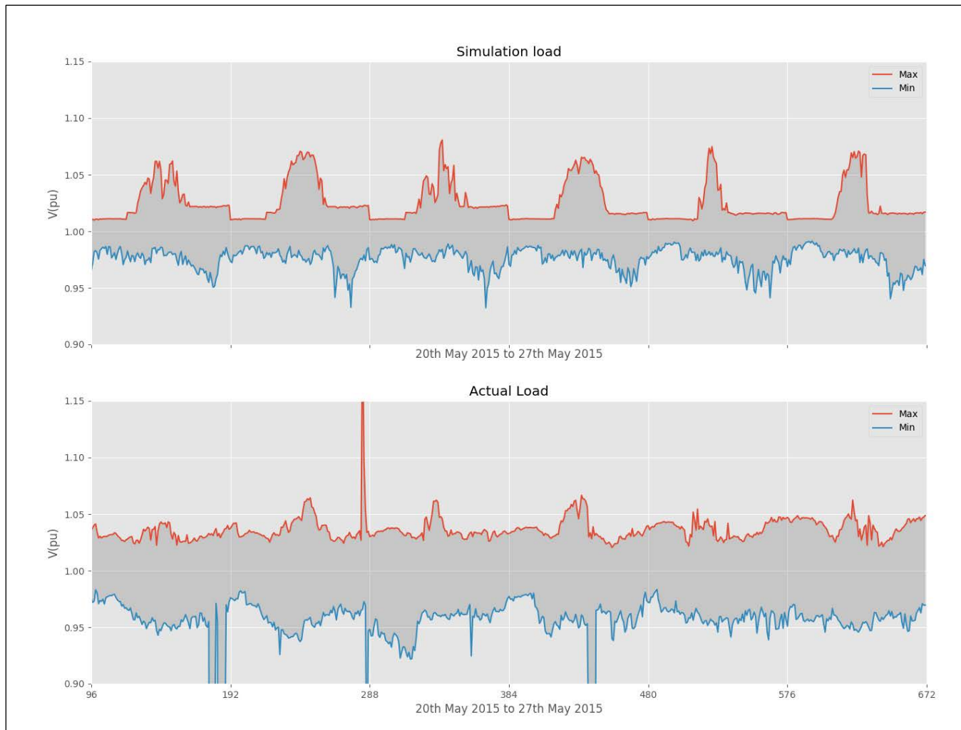
Figure 25. Envelope of maximum and minimum voltages for simulated load (top) and measured AMI loads (bottom) for all customer loads in feeder L.
